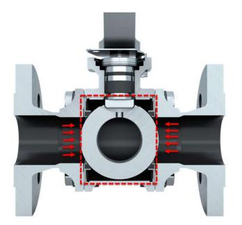
The automatic sealing chamber of the Ballostar KHA ball valve utilizes spring loads in two sealing elements for the function of the valve. The result is an sealing chamber in which the loads of the sealing elements simultaneously **work bidirectionally.** Primarily this concerns safety lines in plants, especially those with alternating flow directions.
